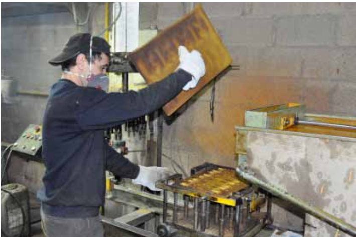
The casting moulds are made from compressed sand
