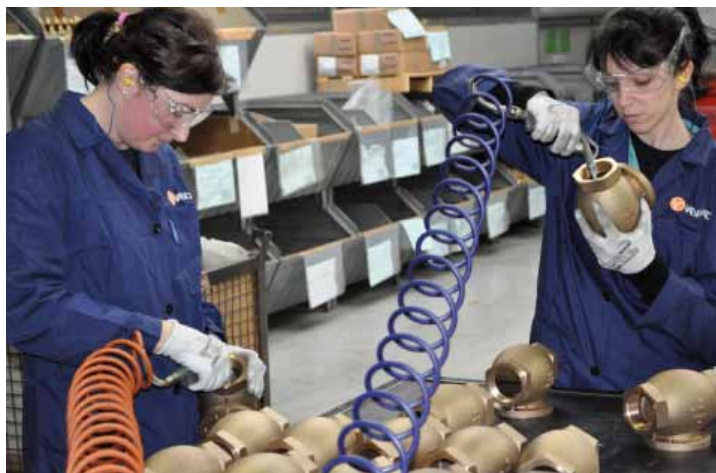
Two employees clean the housings with compressed air
