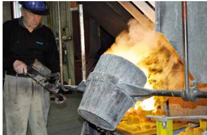
Antonio Campora pours the liquid alloy into the moulds
