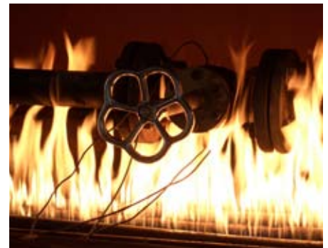
HEROSE LNG cryo valves remain tight even in the event of a fire, in line with the stipulations of EN ISO 10497
