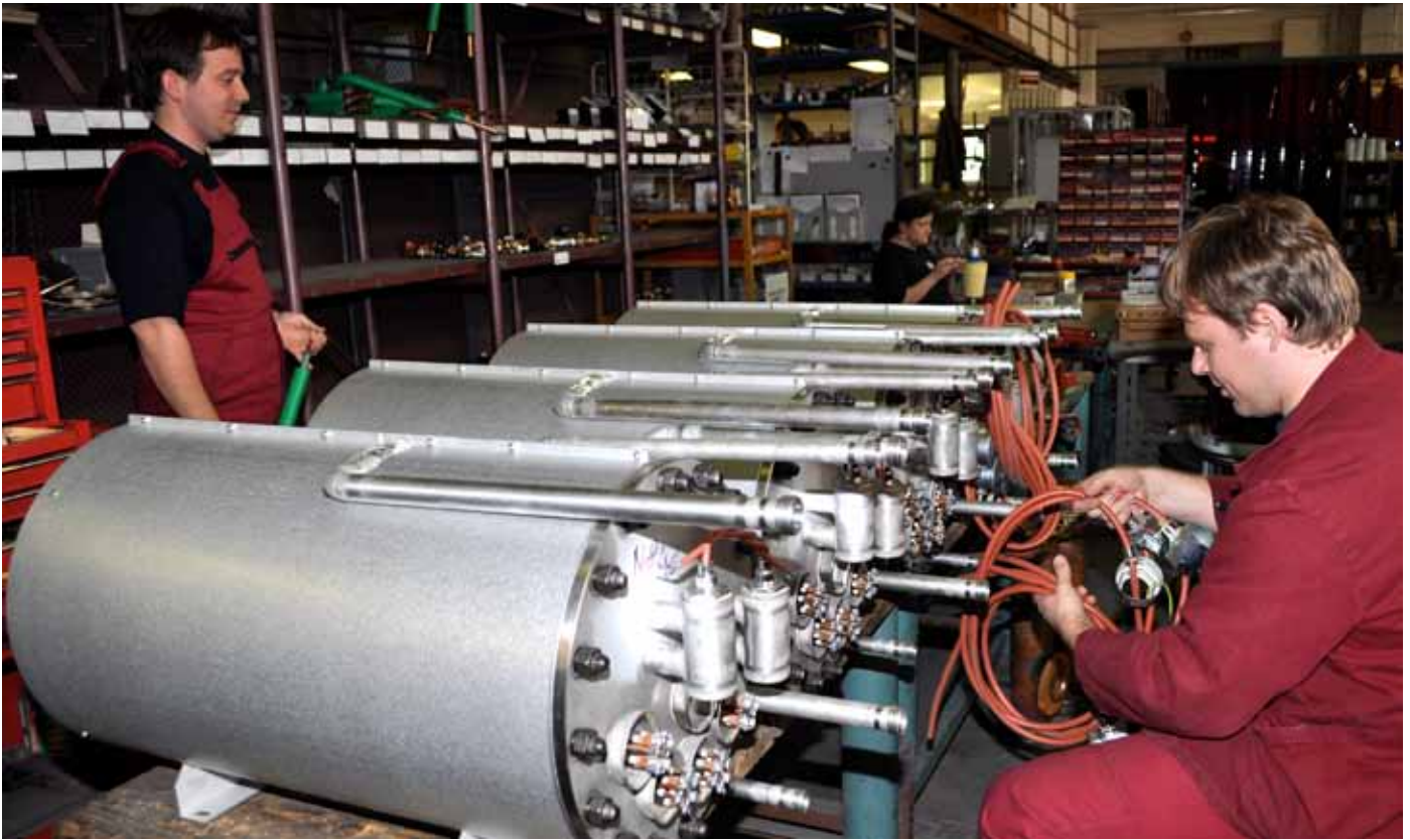
Workers are assembling a pressure container
