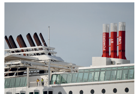
MS Stavangerfjord: on the left the funnels and on the right the "emergency vent" for the LNG tanks
