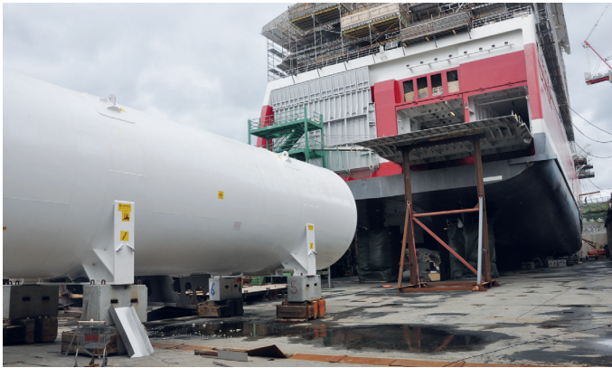
The LNG tank before installation in Rissa, Norway
